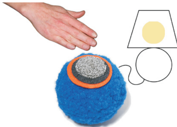
ElectroPUFF Lamp Dimmer, with tufted Plush Touch™ Sensors. © 2006
